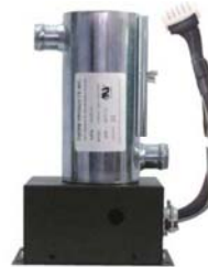
26-08114 4.0KW 240V 9.5" x 3" Maax Spas w/pressure switch, amp plug & cords. 1" barbs Replaces: 26-08115 / 26-08102 26-08116 - 3.0KW Version
